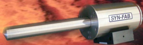
In many boilers and furnaces, variations in fuel infeed and/or combustion air can result in unburned fuel particles being carried up in the flue gas (**carryover**) and deposited on the tubes in the mid to upper furnace areas. These deposits can obstruct gas flow resulting in poor furnace ventilation as well as causing reduced heat transfer. A carryover monitoring system from **SYN-FAB®** can be used as a tool to troubleshoot and resolve such problems.
